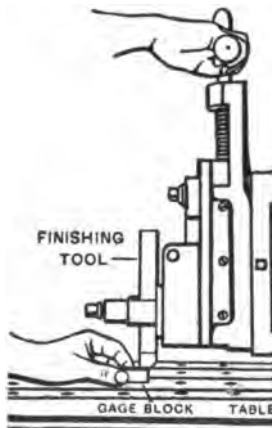
FIG. 25. — GAGE BLOCK TO SET PLANER TOOL.
